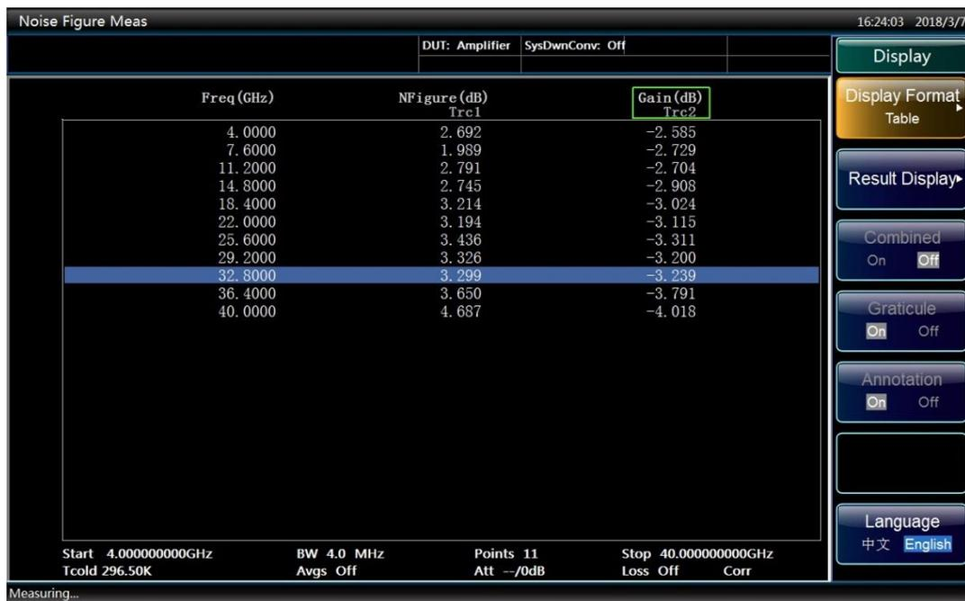
Figure 4.14 Table Display of Measurement Results
