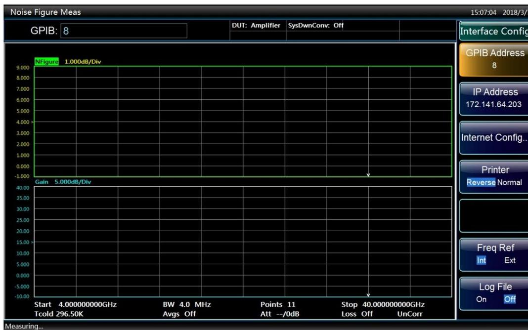
Fig. 3.10 Change GPIB Address
