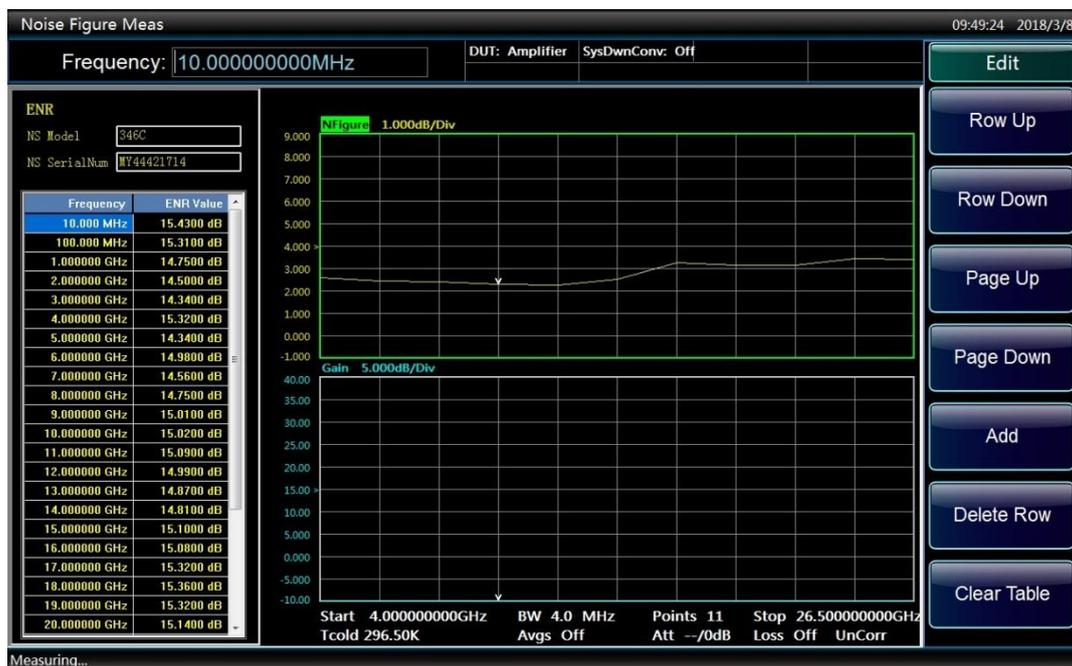
Fig. 3.26 Typical ENR table with entered data
