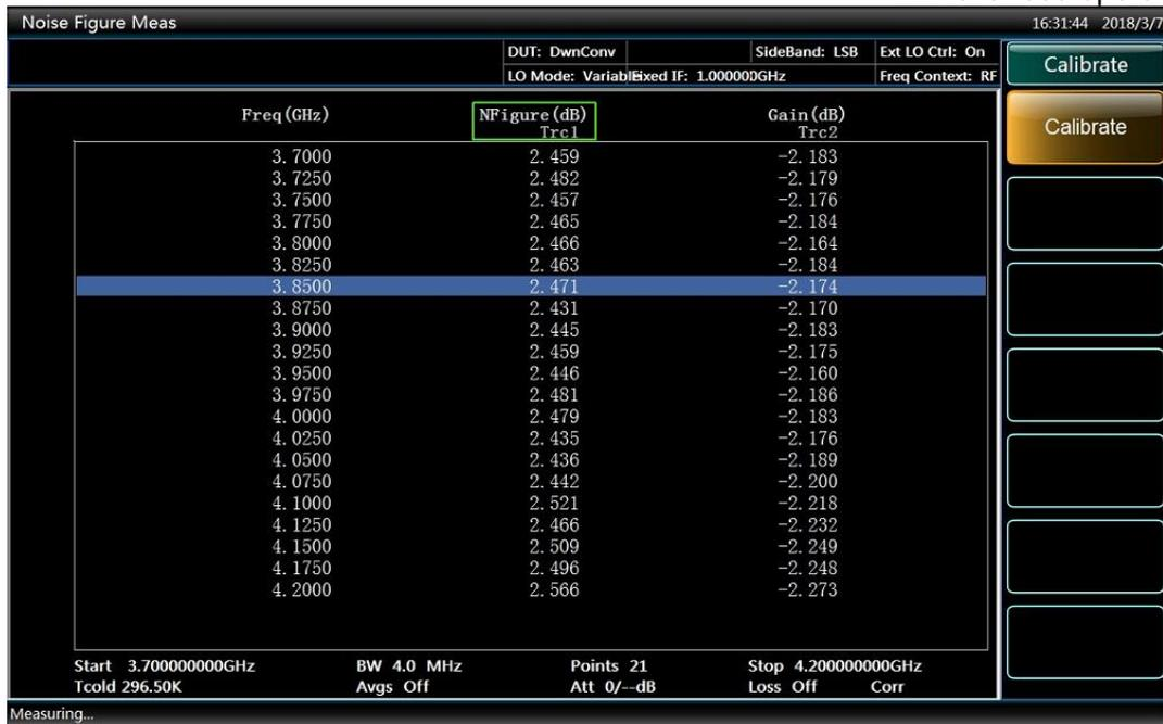
Fig.4.30 Typical measurement values at the downconverter measurement mode
