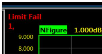
Fig.4.58 Limit Line Failure indicator
