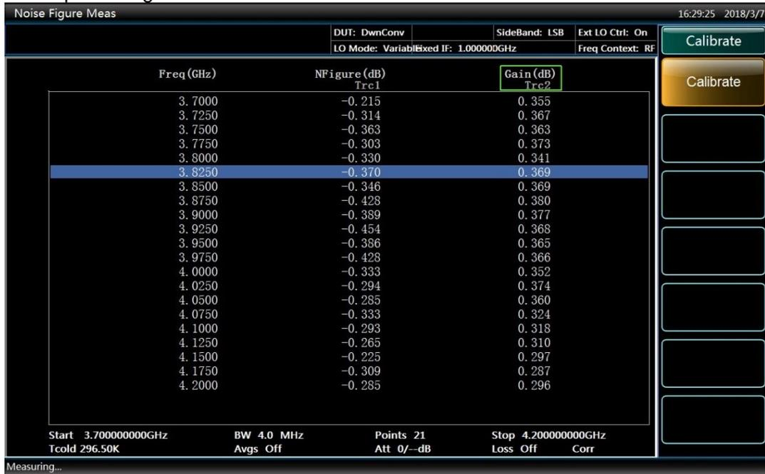
Fig.4.28 Typical calibrated results at the downconverter measurement mode
