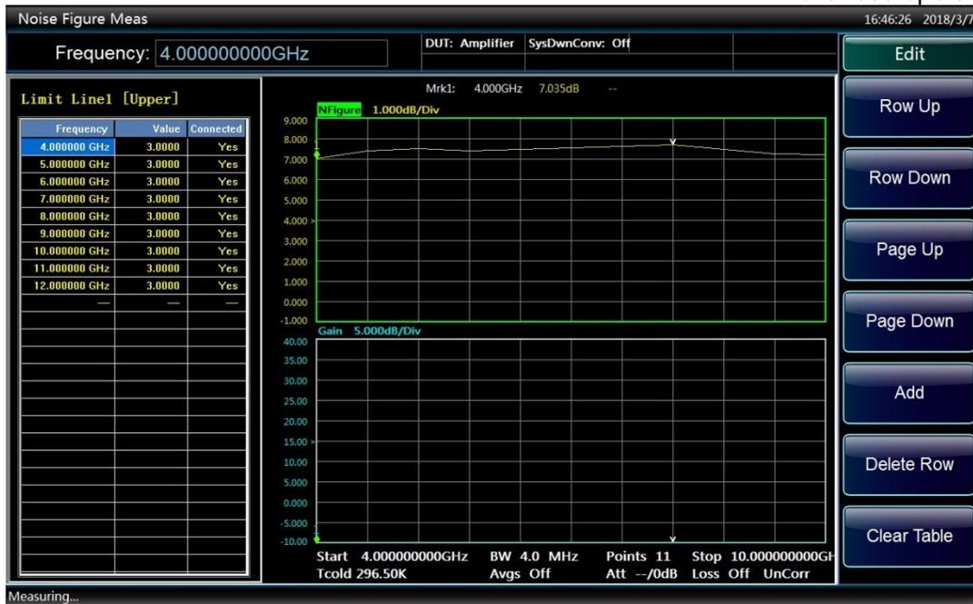
Fig.4.56 Typical Limit Line Table
