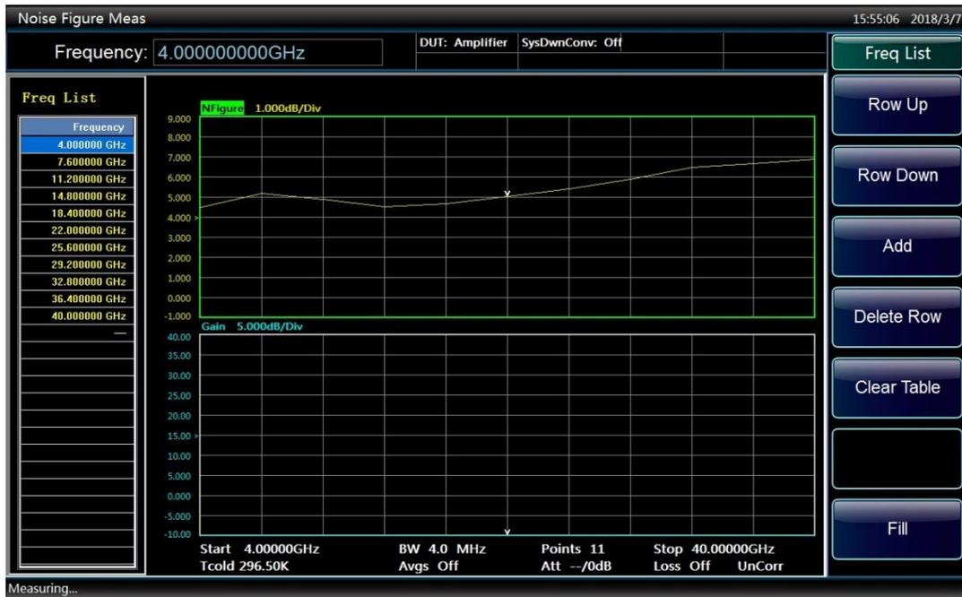
Fig. 3.28 Typical frequency list with entered data
