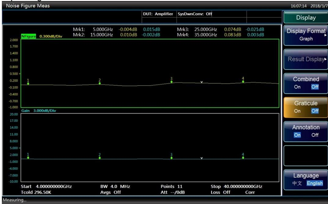
Fig. 3.36 Typical graph display with graticule switched off
