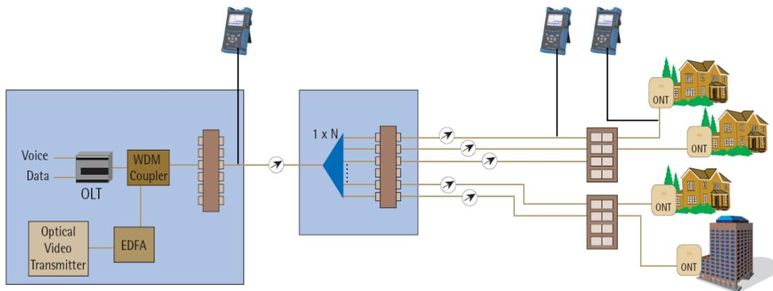
6416 Palm OTDR is mainly used to test FTTH network. It provides a low cost test solution for users. 6416 offers three test modes: manual (real-time, averaging), automatic, and dead zone.
