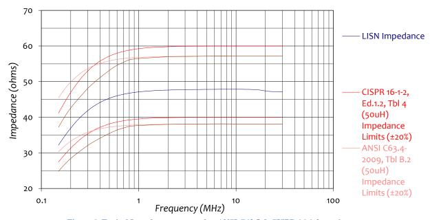
Figure 6: Typical Impedance compared to ANSI C63.5 & CISPR 16-1-2 requirements
