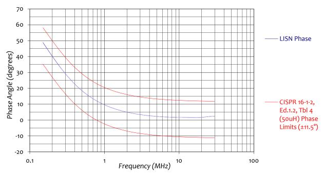
Figure 7: Typical Phase compared to CISPR 16-1-2 requirements.
