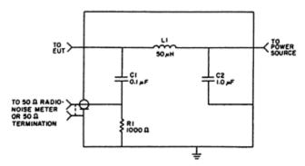
Figure 5: Example of equivalent LISN circuit
