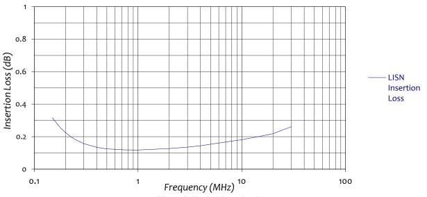
**Figure 9: Typical Insertion Loss**
