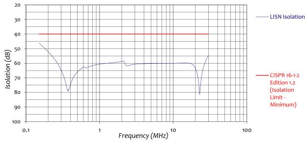
Figure 8: Typical Isolation compared to CISPR 16-1-2 requirements
