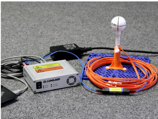
The LSProbe 1.2 system consists of the optically powered E-Field Probe and the Computer Interface shown above. The Computer Interface is connected to the host computer via USB 2.0.
