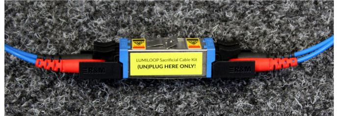
Sacrificial optical cables are supplied with each LSProbe E-Field Probe. Always use the E2000 connectors shown above for breaking and making the optical connection. The E2000 connectors of the sacrificial cable assembly include automatic shutters preventing contamination and resulting optical fiber burn-in. Nevertheless, all optical connectors must be kept in a perfectly clean condition at all times.
