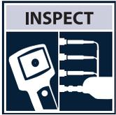
**Inspect First** – Even if you are dealing with a new connector, inspect it with a tool specifically designed for the purpose. You only want to clean the connector if it's necessary
