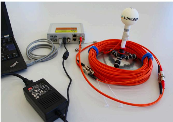
The LSProbe 1.2 system consists of the optically powered E-Field Probe and the Computer Interface shown above. The Computer Interface is connected to the host computer via USB 2.0.
